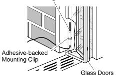
Figure 35 - Installing Thermostat Sensing Bulb behind Glass Doors
